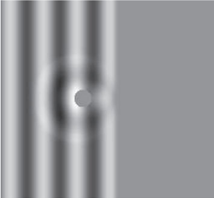
TLM simulation of plane wave scattered by a circular scatterer.
