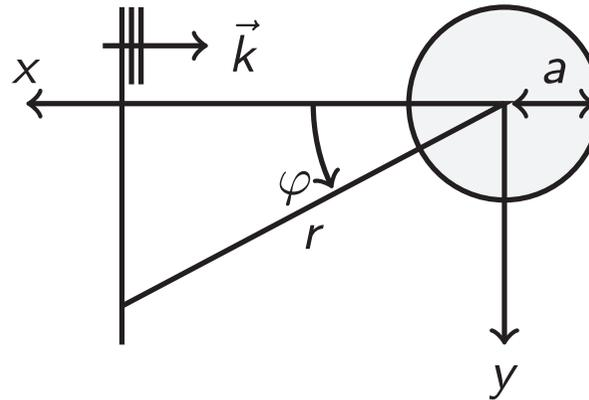
Schematic of wave propagation in the vicinity of a cylinder.
