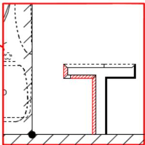
**Absorbent: D&B layer –  $\sigma = 50 \text{ kPa s/m}^2$ ,  $d = 10 \text{ cm}$**
