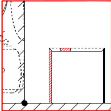
20 Absorbent: D&B layer –  $\sigma = 50 \text{ kPa s/m}^2$ ,  $d = 10 \text{ cm}$
