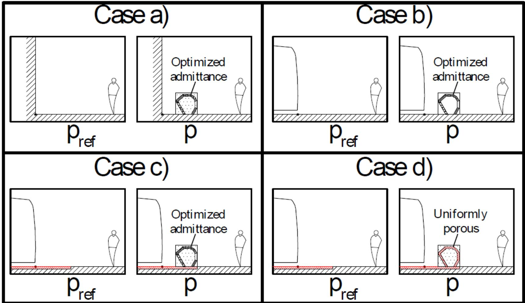
**Absorbing ground : Delany & Bazley layer –  $\sigma = 50 \text{ kPa s/m}^2$  ,  $d = 10 \text{ cm}$**
