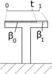
Gradient with respect to a panel width
