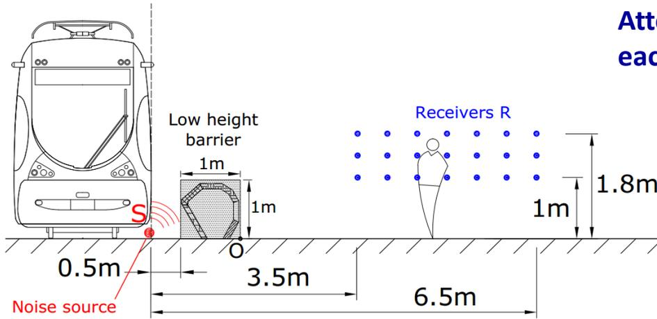
Attenuation at each frequency  $A_n = \left[ \frac{\sum_i |p(R_i, f_n)|^2}{\sum_i |p^{in}(R_i, f_n)|^2} \right]^{\frac{1}{2}} = \frac{P(f_n)}{P^{in}(f_n)}$
